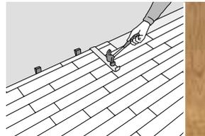
After the last board is in place, all wedges must be removed. The expansion gaps are then covered with moldings. They must allow natural expansion and movement of the floor.
