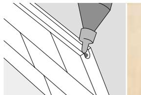
Join the elements immediately using a square edged hardwood tapping block (1 ft. or longer) and a hammer. The tapping block should always be positioned along the tongue.
