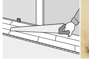
If the door jamb cannot be cut, maintain an expansion gap. It can be covered with elastomeric sealer or a wooden profile (molding).
